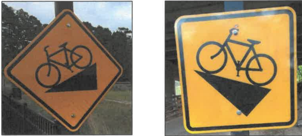
Figure 7: W7-5 Bicycle hill warning signage
